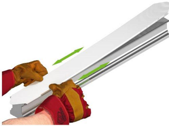
Fig. 5.27: Mounting the cover strip
