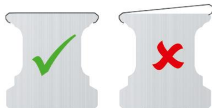
Fig. 5.45: Correctly and incorrectly fitted cover strip
