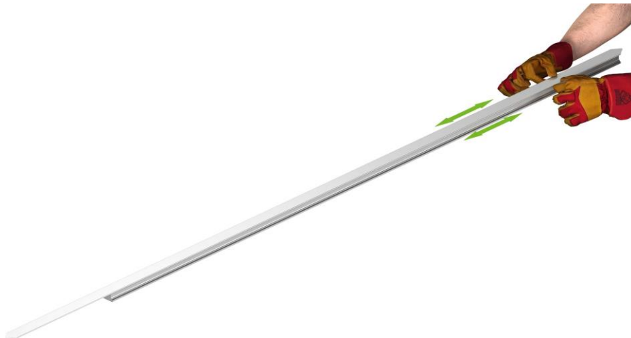
Fig. 5.28: Clamp on cover strip approx. 3 cm
